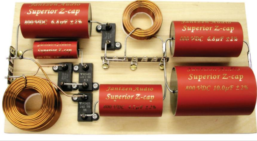
**Please note!** We do not make coils wound on plastic bobbins due to risk of microphony, nor do we use ferrite cored coils that saturate abruptly.
