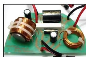
**Please note!** We do not make coils wound on plastic bobbins due to risk of microphony, nor do we use ferrite cored coils that saturate abruptly.
