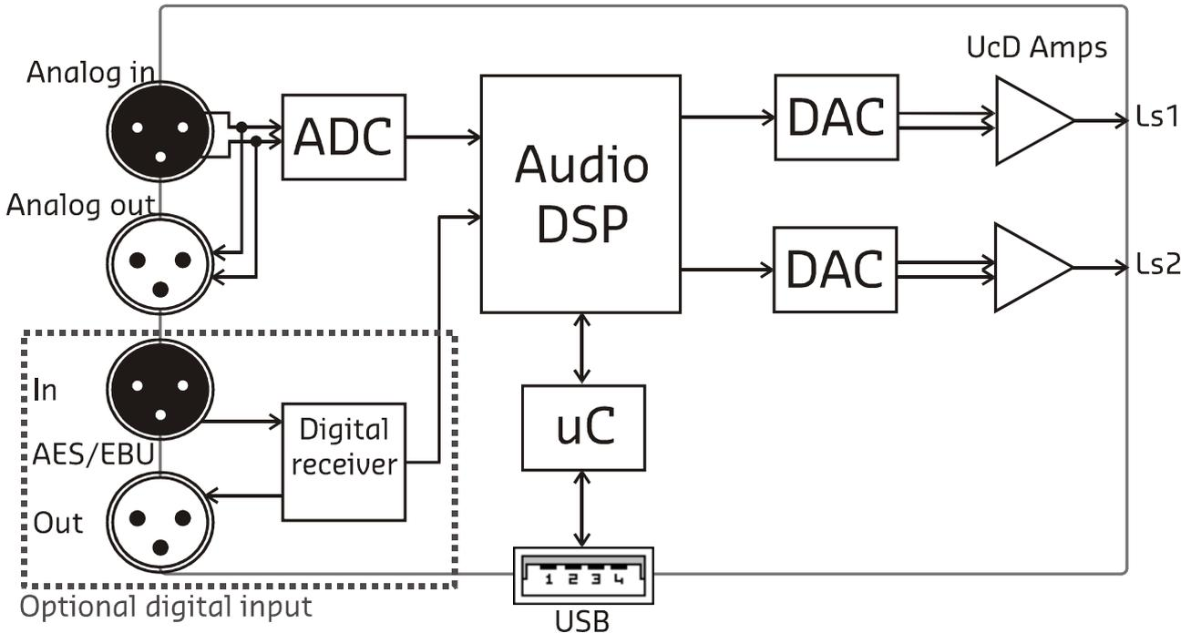
Figure 4: Block diagram
