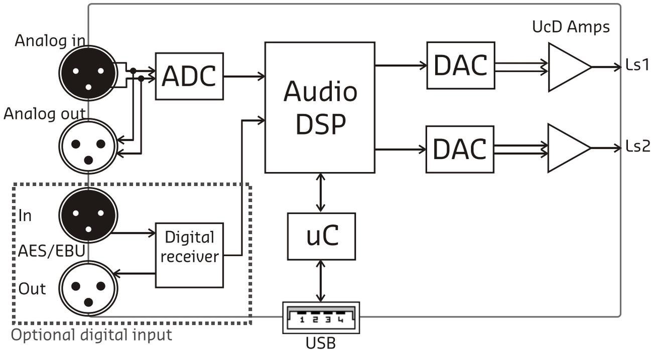
Figure 3: Block diagram
