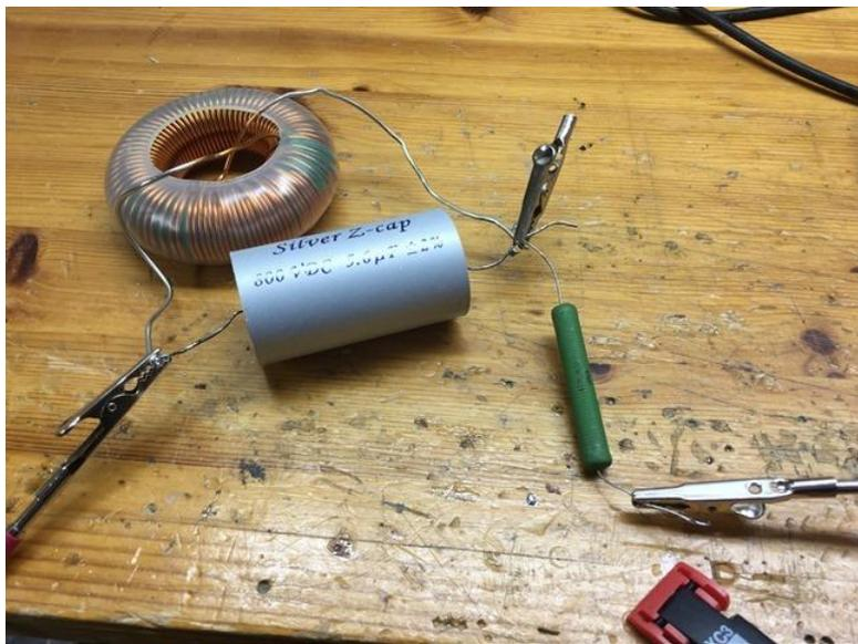
Then you do the impedance measurement, i.e. 100-5000 Hz, depending on the capacitors value (in this example a 5.6 uF was used).
