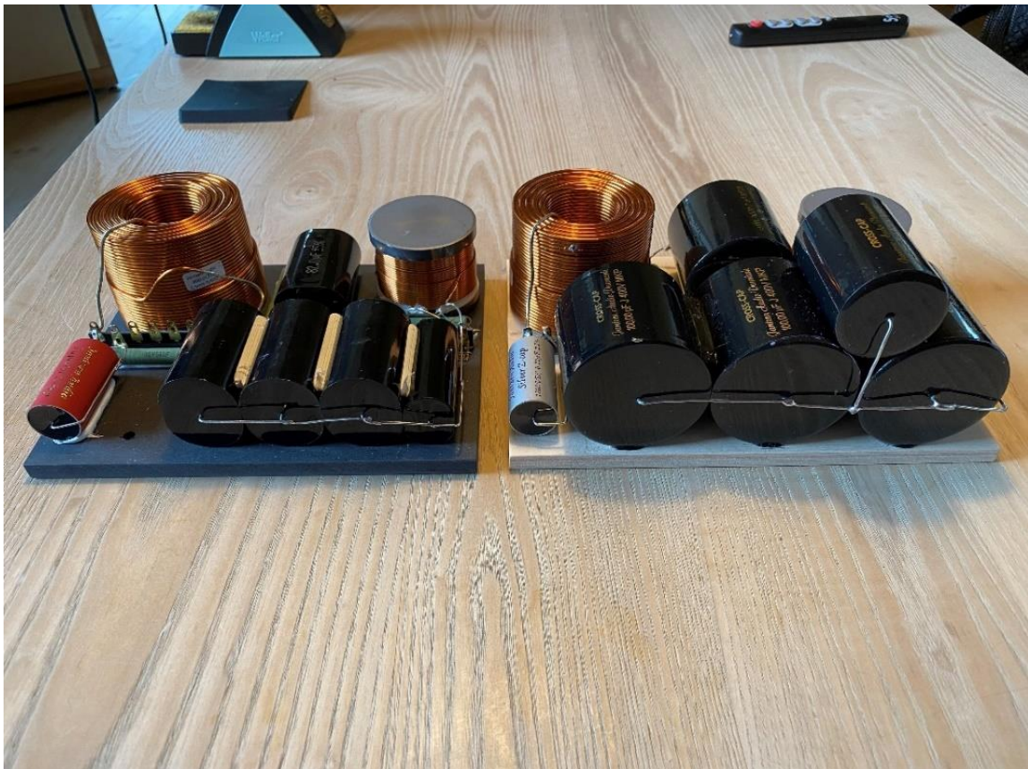
347 \mu F in parallel, MKT Z-caps on the left and Cross Caps on the right
