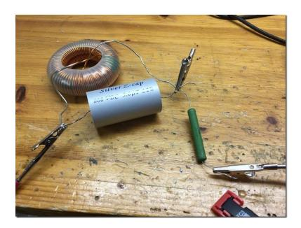
1.) Do the impedance measurement, i.e. 100-5000 Hz, depending on the capacitors value (in this example a 5.6 uF was used).
